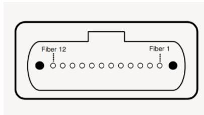
Figure 2 Optical connector
