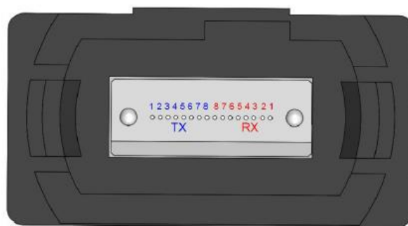
Figure 3. MPO-16 Optical connector Interface
